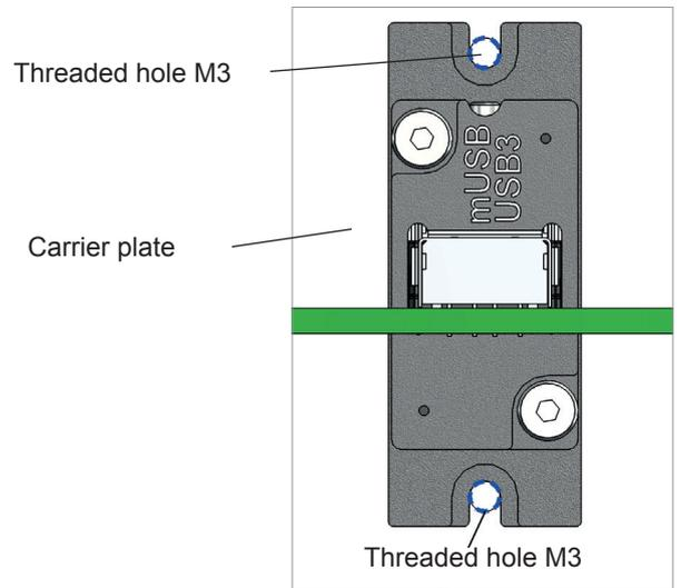
Cut a sufficient opening into the carrier plate to have enough space for later insertion of the test connector from the back. Leave at least 1 mm space between opening and test connector.
