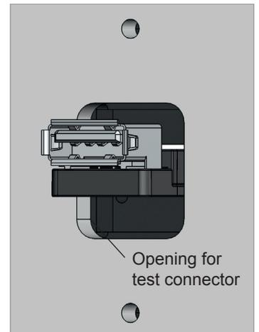
Loosen the retaining screw of the test connector. Insert the test connector into the DUT until it comes to rest. Retract the test connector for 0.5 to 1 mm in order to prevent damages of the DUT.
