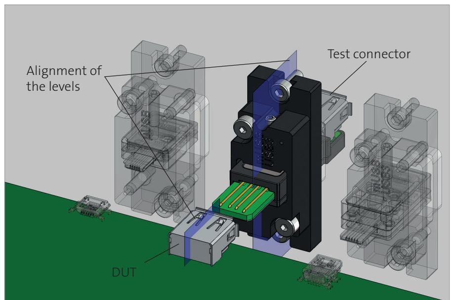
Align the lower level of the test connector on the lower internal level of the connector to test (DUT)
